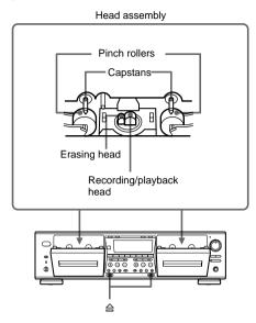
Clean the heads and tape path of the tape deck after every 10 hours of operation to guard against:
